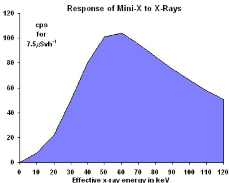
N.B. Above response curve for MX168 geiger tube with protective plastic cap fitted.
